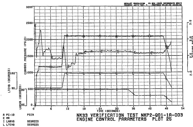
Figure 14. Performance Parameters for Verification Test #003
