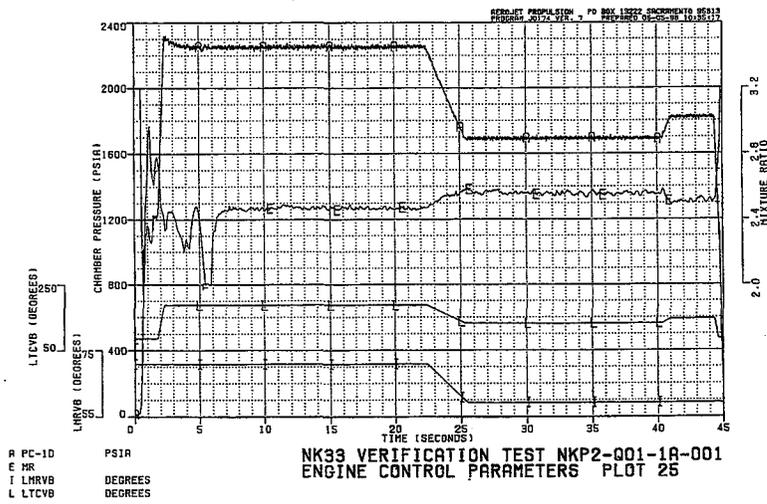
Figure 12. Performance Parameters for Verification Test #001
