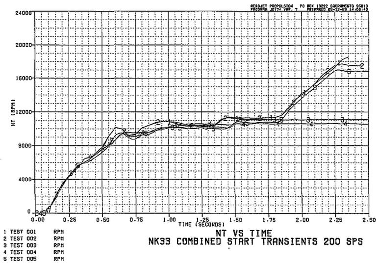
**Figure 19. Verification Test Start Transient Comparison of Turbopump Shaft Speeds**
