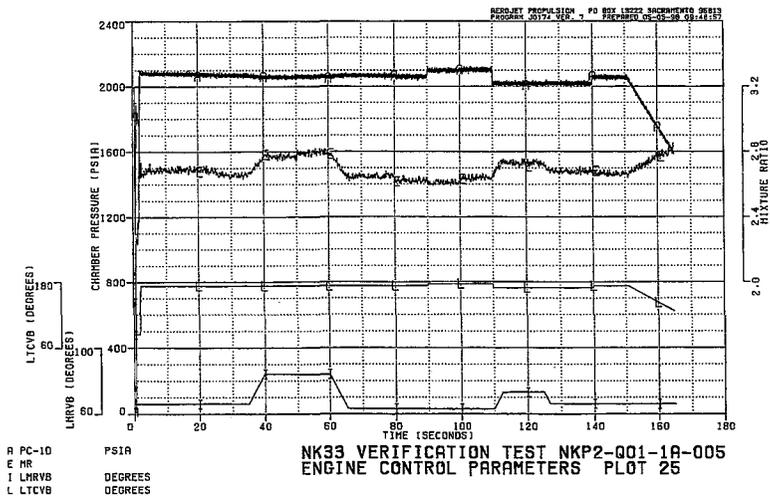
Figure 16. Performance Parameters for Verification Test #005
