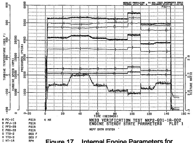
Figure 17. Internal Engine Parameters for Verification Test #002
