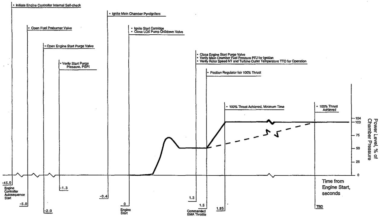
Figure 8. Start Transient of the Modified NK-33 Engine (AJ26-58, 59)
