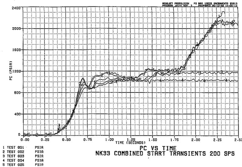
Figure 18. Verification Test Start Transient Comparison of Main Combustion Chamber Pressures
