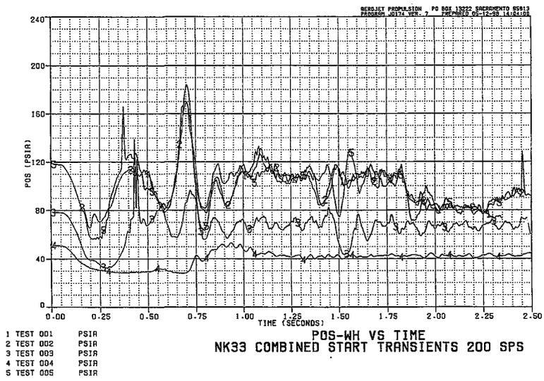
**Figure 20. Verification Test Start Transient Comparison of Oxidizer Inlet Pressures**
