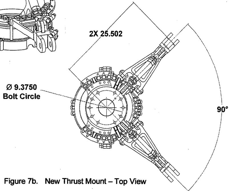
Figure 7b. New Thrust Mount – Top View
