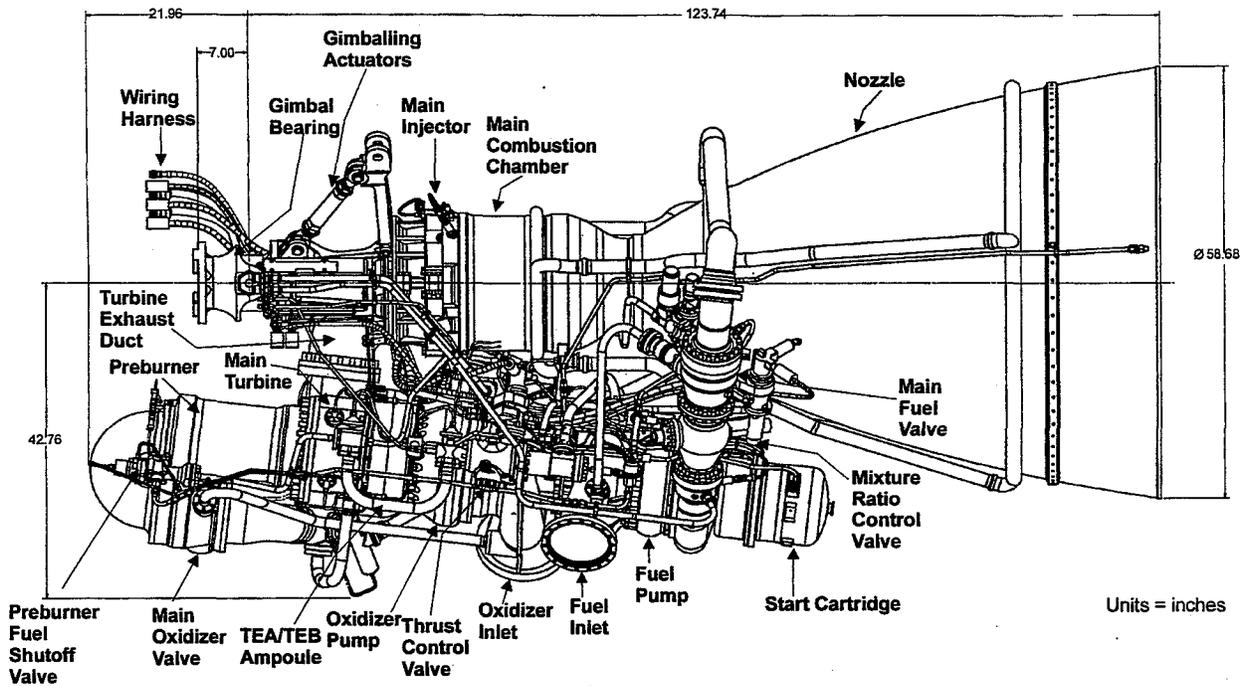
Figure 3. Layout Envelope of the Modified Basic NK-33 Engine (AJ26-58) - Side View
