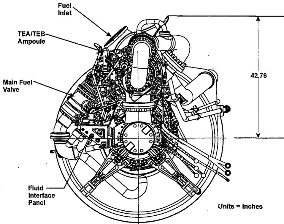
Figure 4. Layout Envelope of the Modified Basic NK-33 Engine (AJ26-58) - Top View
