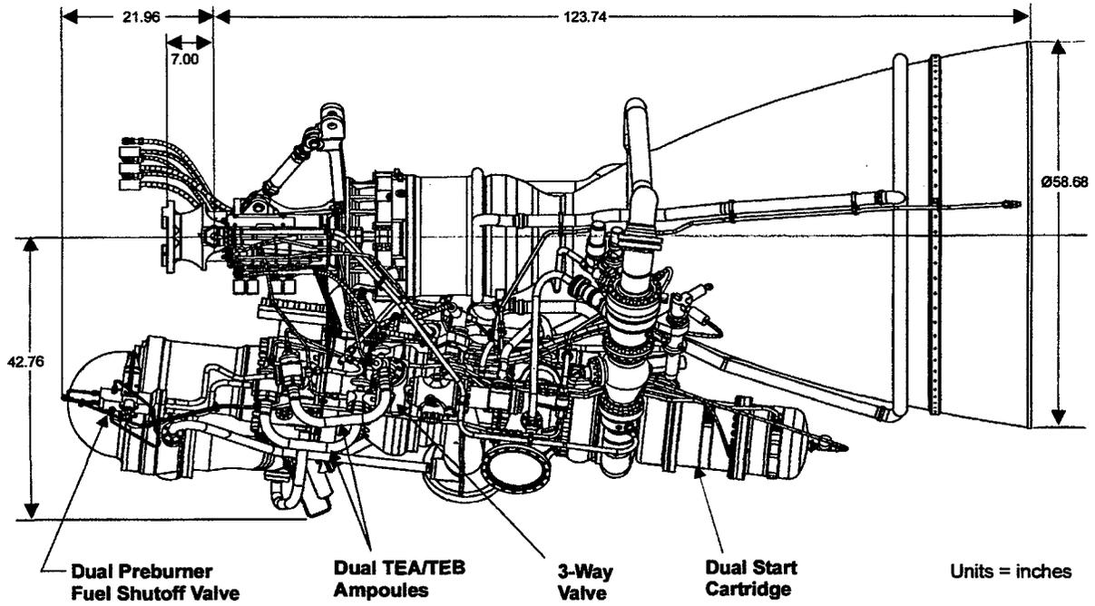
Figure 5. Layout Envelope of the Modified Restartable NK-33 Engine (AJ26-59) - Side View
