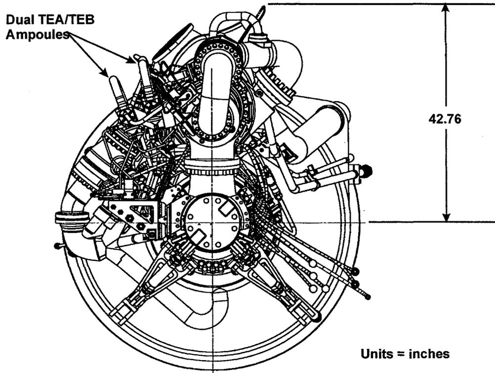
Figure 6. Layout Envelope of the Modified Restartable NK-33 Engine (AJ26-59) - Top View
