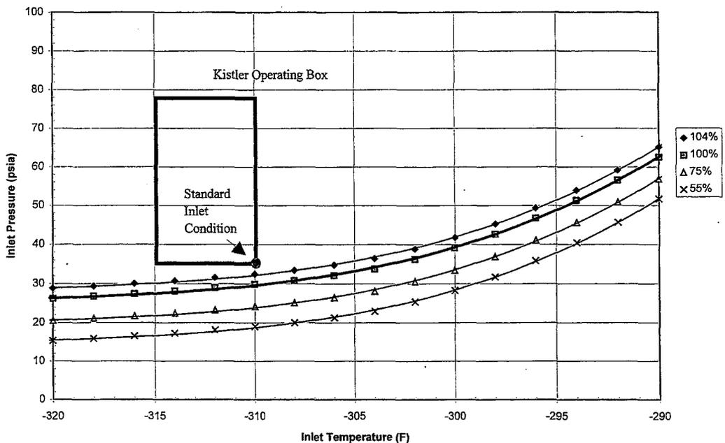
Figure 10. LOX Engine Inlet Pressure and Temperature for Modified NK-33 Engines (AJ26-58, 59)
