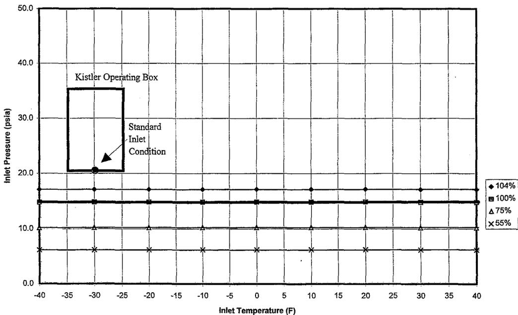
Figure 9. RP-1 Engine Inlet Pressure and Temperature for Modified NK-33 Engines (AJ26-58, 59)
