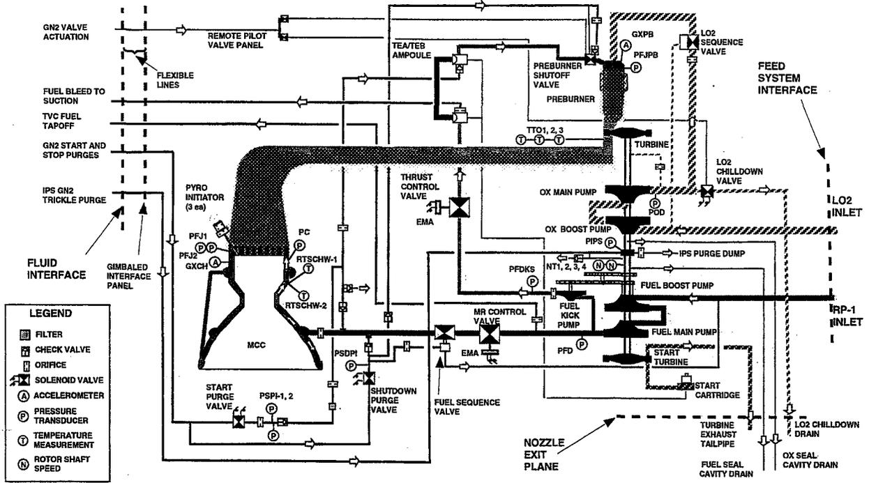
Figure 1. Schematic of the Modified Basic NK-33 Engine (AJ26-58)
