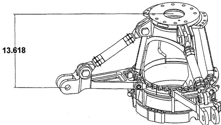
Figure 7a. New Thrust Mount – Side View
