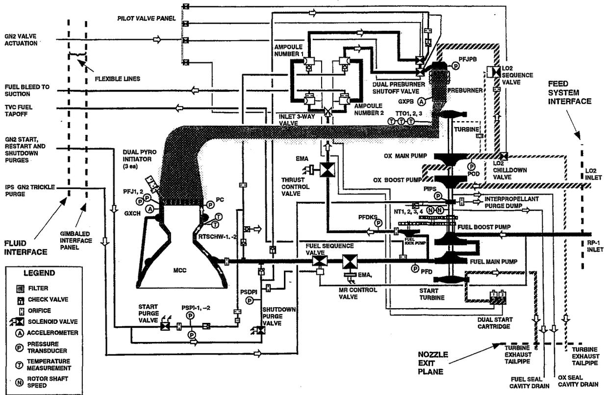
Figure 2. Schematic of the Modified Restartable NK-33 Engine (AJ26-59)
