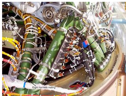
Figure 18. The RD-180 Electrical Interface Mated to the Vehicle
