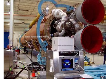
Figure 17. Electrical Testing on the RD-180 using the ETU (foreground)
