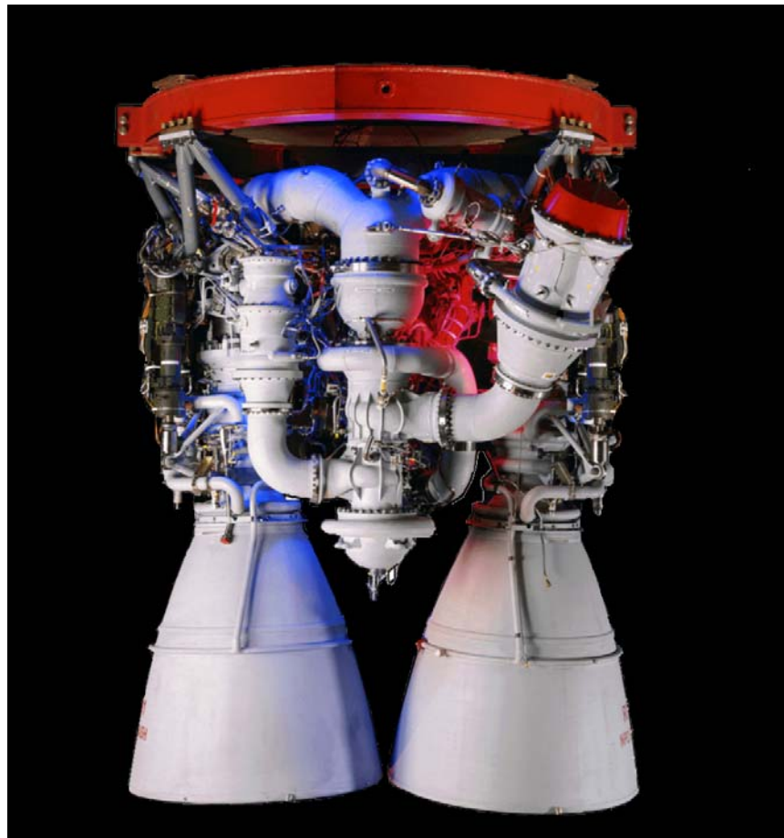
Figure I-1 RD-180 Engine 4A Shown Mounted to Handling Frame
