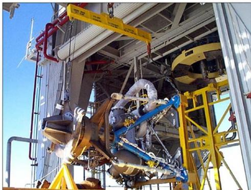
Figure 19. Turbomachinery Power Pack Risk Reduction Testing
