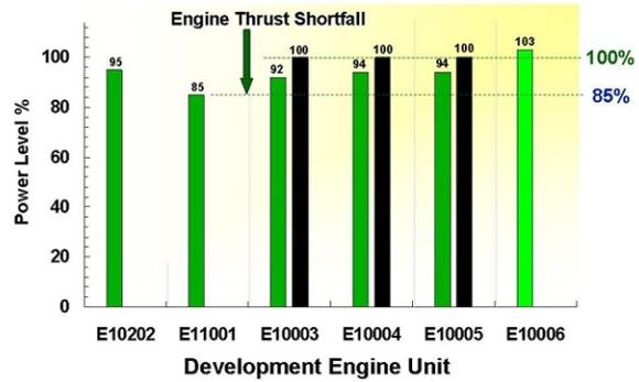
**Figure 35. Engine Thrust Shortfall**
